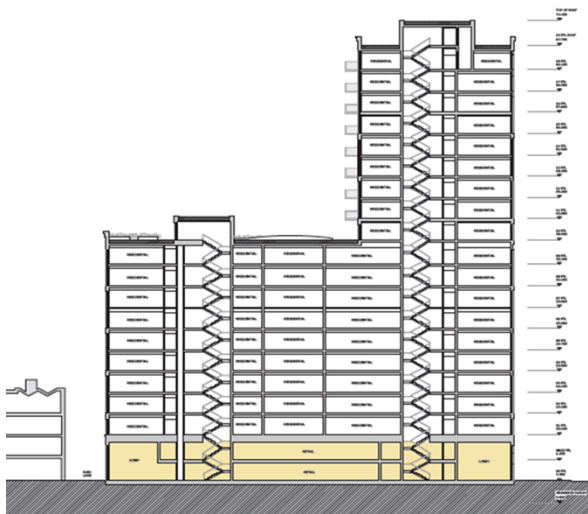
Image: Section showing retail and commercial at ground, mezzanine and first floor levels
